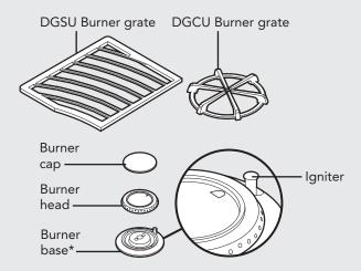
\*Note: When replacing burner head, carefully align the tab underneath the cap with the slot in the burner base.
